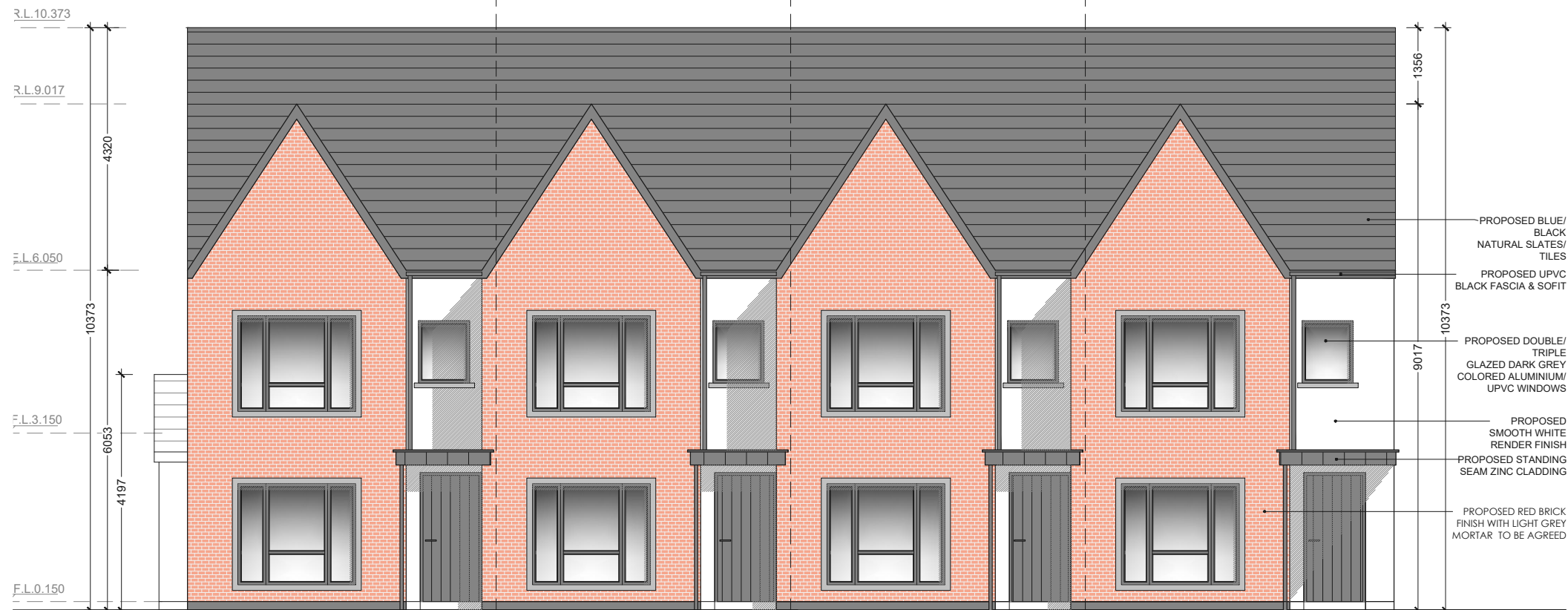
TYPE D2 - PROPOSED 3 BED TERRACED FRONT ELEVATION - SCALE 1:100
