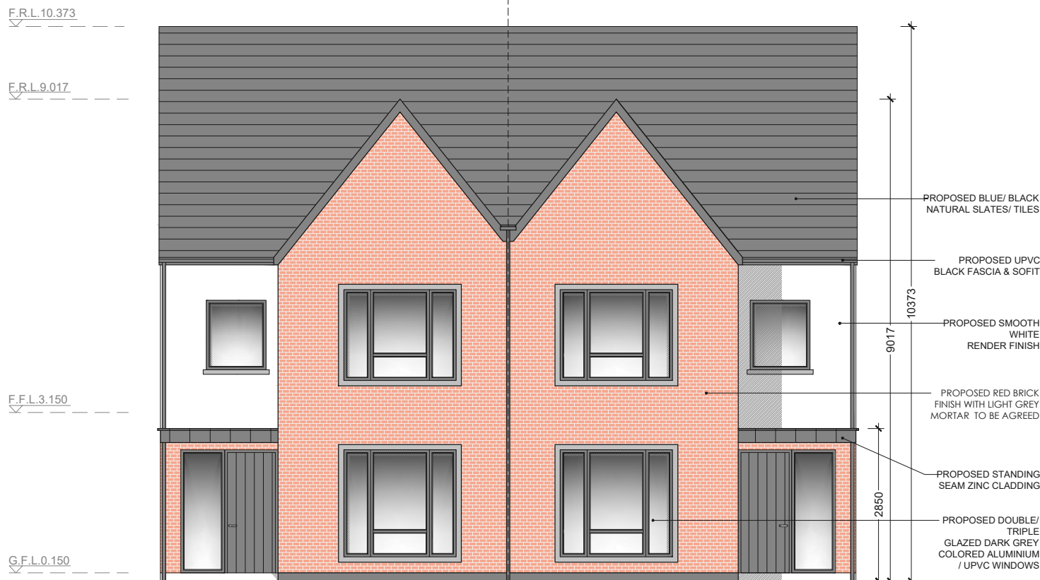
TYPE C2 - PROPOSED 3 BED SEMI-DETACHED DWELLINGS FRONT ELEVATION - SCALE 1:100
