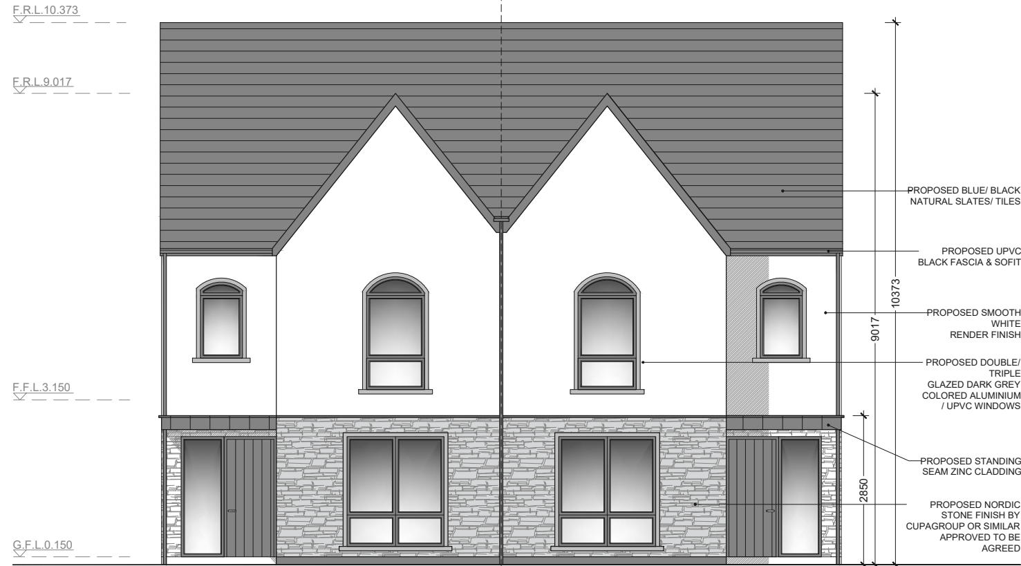
TYPE C1.1 - PROPOSED 3 BED SEMI-DETACHED DWELLINGS FRONT ELEVATION - SCALE 1:100
