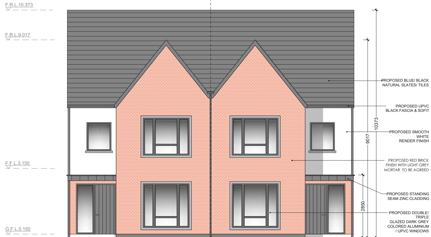
TYPE C1 - PROPOSED 3 BED SEMI-DETACHED DWELLINGS FRONT ELEVATION - SCALE 1:100
